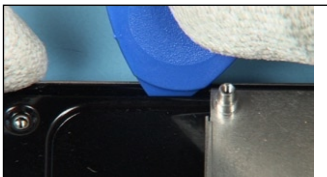
36. Slightly open the clips of the SLIDE MODULE ASSY.
